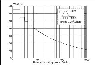
Fig.4. Maximum permissible non-repetitive peak on-state current  $I_{TSM}$ , versus number of cycles, for sinusoidal currents, f = 50 Hz.
