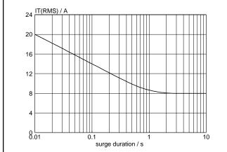
Fig.5. Maximum permissible repetitive rms on-state current  $I_{T(RMS)}$ , versus surge duration, for sinusoidal currents, f = 50 Hz;  $T_{mb} \le 107$  °C.
